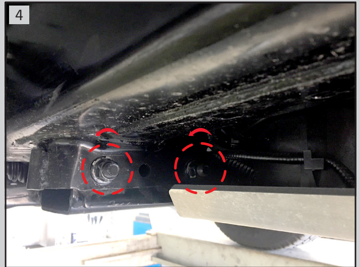
Front left bracket (B1): Open 2 Nuts
