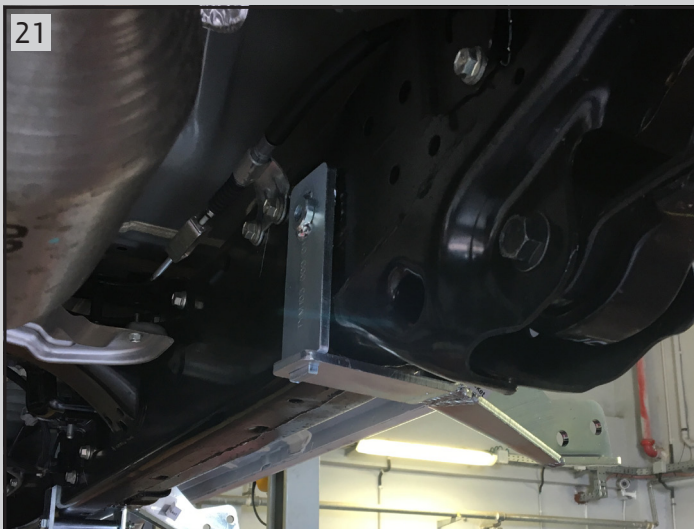
21 Place bracket (D2+D4) on chassis
