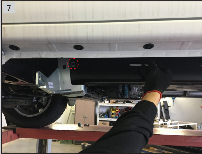
7 Place bracket (B1) and insert plate (B3). Align the plate to the hole
