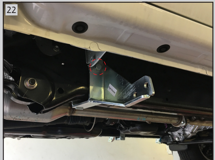
22 Connect bracket (D2+D4) to chassis using hex bolt (E), spring washer (H) and washer (G)
