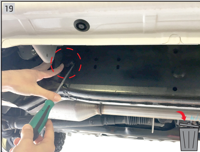
19 Rear right bracket: Remove the cap on chassis outer side
