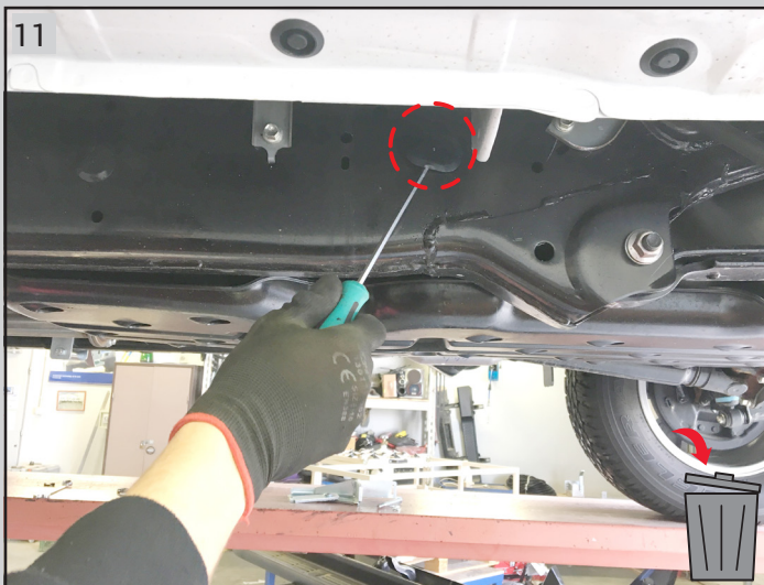
11 Rear left bracket (D1): Remove the cap
