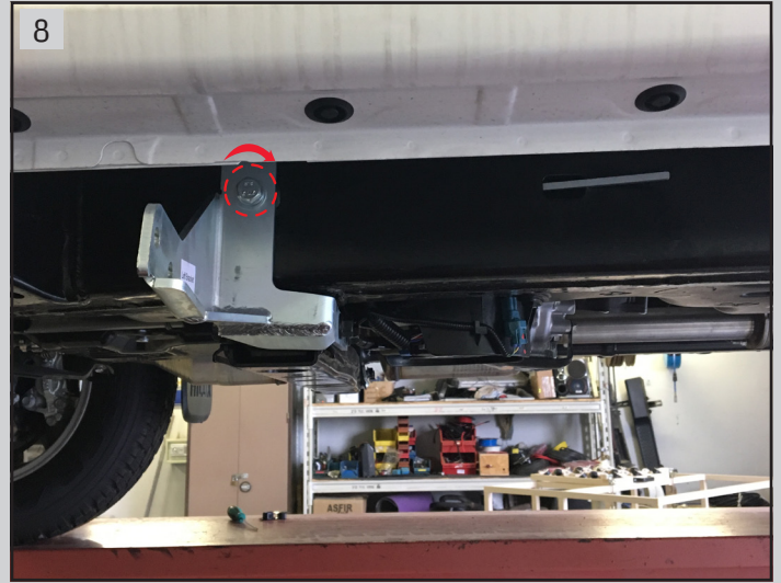
8 Connect bracket (B1) to chassis using bolt (G), spring washer (H) and hex bolt (I)
