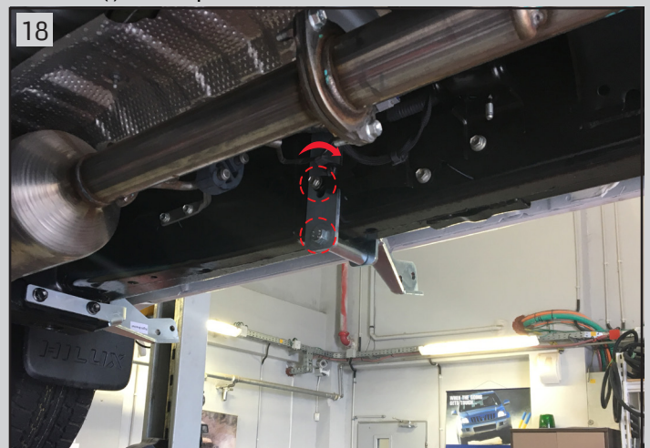
18 Connect bracket (C2+C4) to chassis using original bolt. Insert spacer (F) and tighten bolt (I) and hex nut (J)
