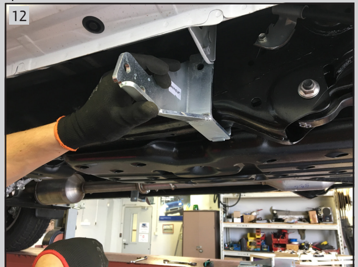
12 Connect bracket (D1+D3) to chassis using hex bolt (J) washer (G) and hex nut (I)
