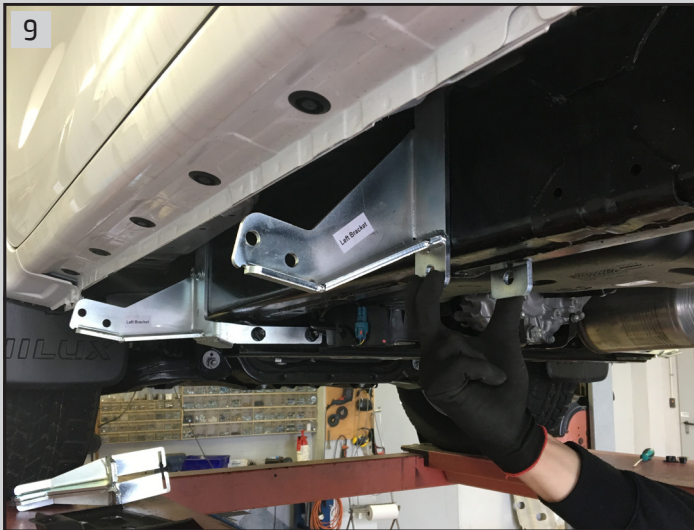
9 Middle left bracket (C1+C3): Place bracket on chassis
