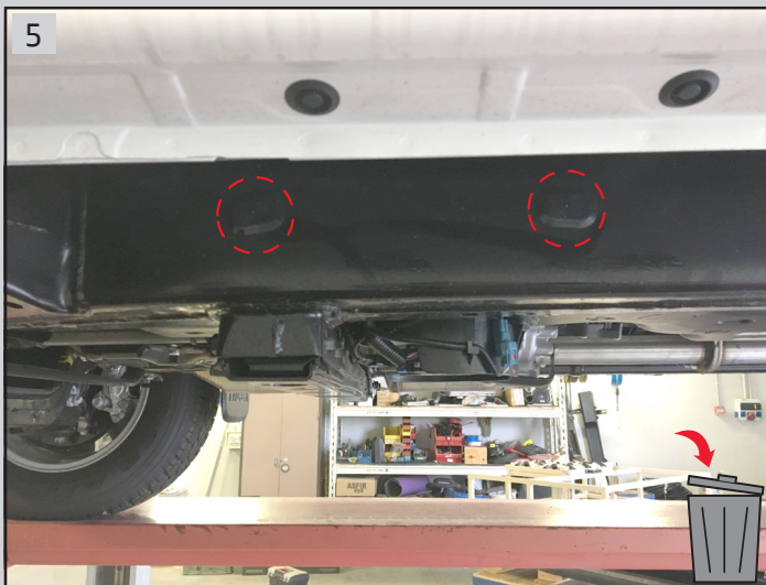
Remove 4 caps. 2 on right side of the vehicle. 2 on left side of the vehicle
