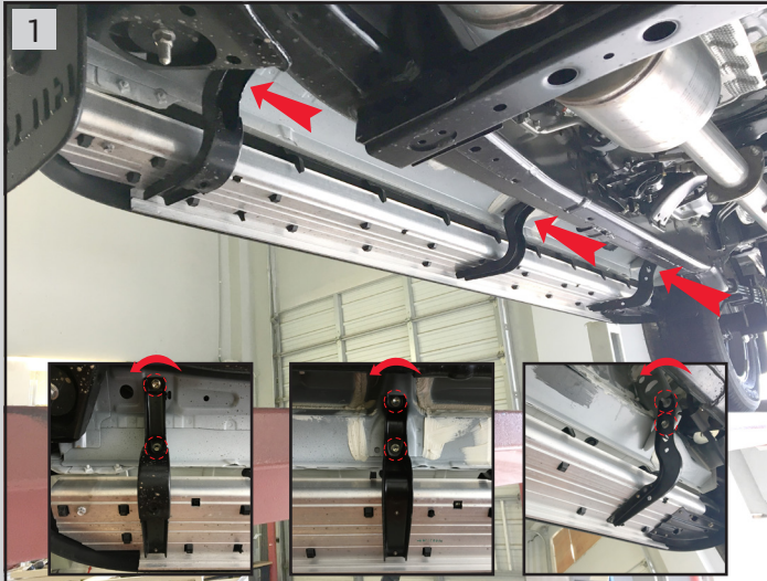
Remove bolts and dispose the original step
