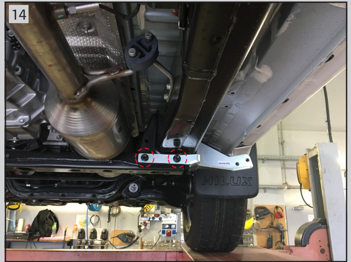
14 Install bracket (B2) with the original nuts
