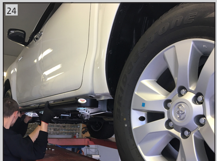
24 Place right and left steps (A1+A2) on the brackets and place hex bolts (I), hex nut (J) and washer (G)
