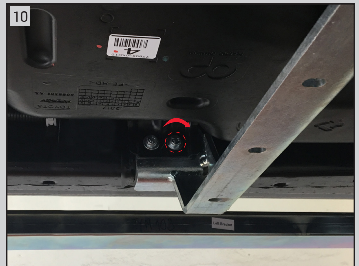
Tighten Right bolt (H)
