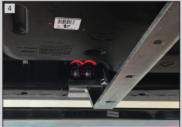
4 Connect bracket (B) left side to the chassis using bolt (H), spring washer (M) and washer (K). Right bolt - dont tighten it yet, leave for after placing the skid plate
