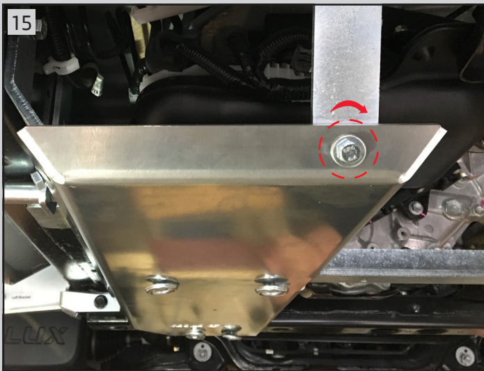
Connect plate (A) to bracket (C) using bolt (I), washer (L- on both sides of the plate) and hex nut (K)
