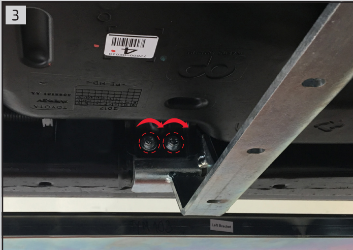
3 Place bracket (B) and connect it using bolt (H), spring washer (M) and washer (K) to the chassis. Right bolt - dont tighten it yet, leave for after placing the skid plate
