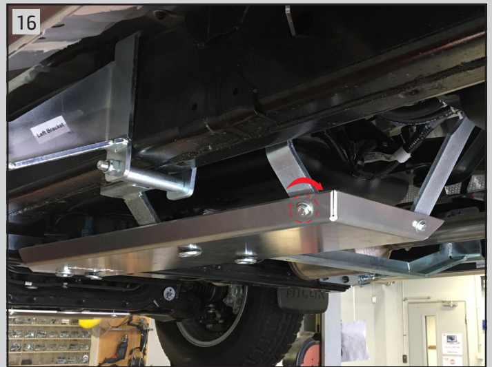
Connect plate (A) to bracket (D) using bolt (I), washer (L- on both sides of the plate) and hex nut (K)
