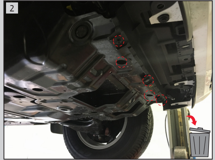
2 Remove 4 bolts and middle clips. Dispose the original plate
