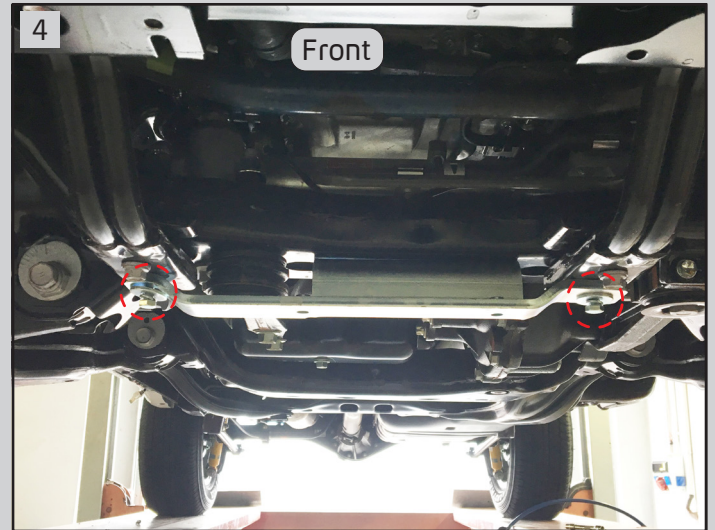
4 Connect the bracket to the original screwing using hex bolt (E), spring washer (I), and washer (G)
